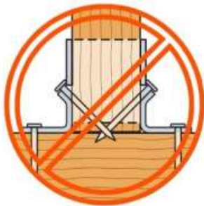
10dx1 1/2" nails may not be used as double shear nails
